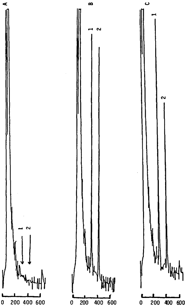
Fig. 1. Gas chromatograms of (A) blank plasma, (B) calibration standard (blank plasma spiked with 5000 ng/ml chlorproethazine and chlorpromazine) and (C) plasma collected 30 min after intramuscular injection of 25 mg of chlorproethazine to a monkey. Peaks: 1=chlorpromazine; 2=chlorproethazine. Time in seconds.
